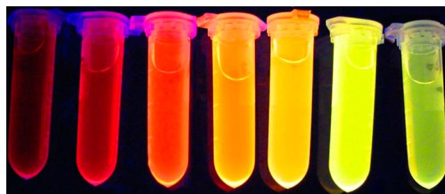
Figure 3. Digital photographs of the \text{CuInS}_2/\text{ZnS} NCs under excitation at 365 nm UV (3:4, 1:2, 3:8, 1:3, 1:4, 1:5, and 1:10).
